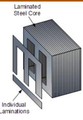
Constructed from laminations of Silicon steel assembled together to provide continuous magnetic path
